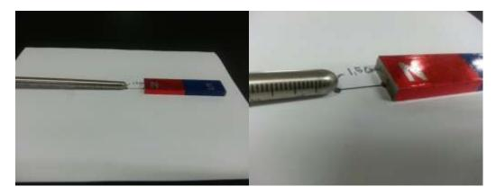
2. Press the button to measure the force of the North pole and record the position. Example: North pole...
