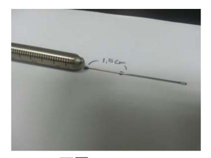
3. Press the button to measure the magnetic force at the needle tip and record the position. Example: Needle tip.
